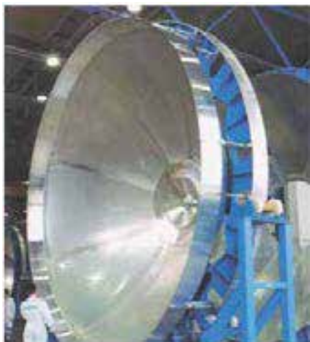
Fig. 4.7: An impressive example of an EB-welding application. In a huge vacuum chamber two 70-mm-thick aluminium plates, with a diameter of 6 metres, are joined with a 'single-shot'. It is the basic material used in forging and machining the main stage of Ariane-rocket tanks.
