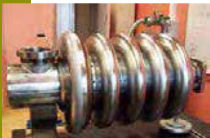
Fig. 2.7: Superconducting accelerating cavities (credit: CEA).
