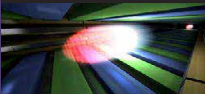
Fig. 7.6: Extremely short and intense X-ray pulses are generated by the long undulator in a SASE FEL (credit: European XFEL/ Marc Hermann).
