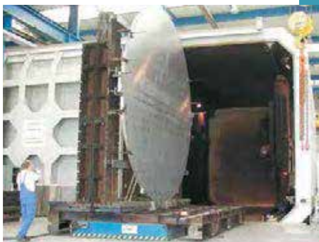
Fig. 4.7: An impressive example of an EB-welding application. In a huge vacuum chamber two 70-mm-thick aluminium plates, with a diameter of 6 metres, are joined with a 'single-shot'. It is the basic material used in forging and machining the main stage of Ariane-rocket tanks.
