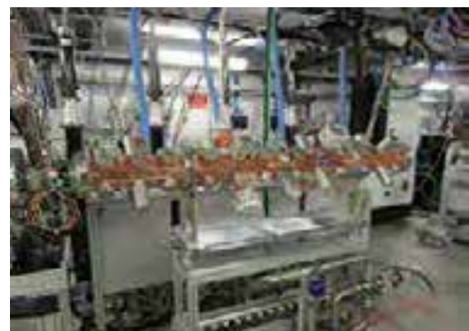
Fig. 2.9: More compact linear accelerating structures are being developed for medical use (credit: CERN).
