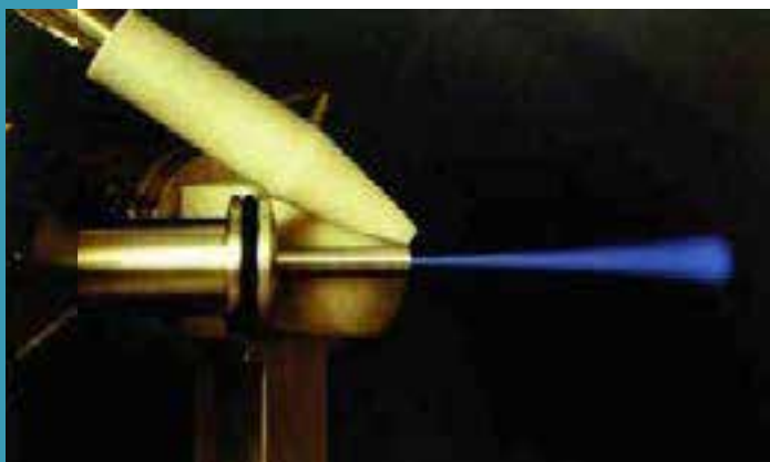
Fig. 4.18: A 3-MeV proton beam extracted into air.
